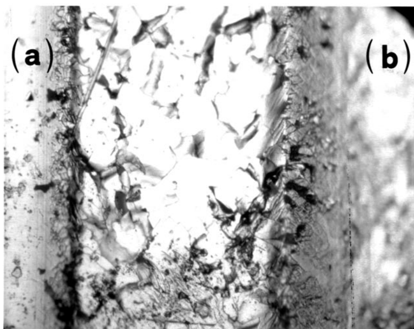
Figure 5. An optical micrograph of scratches on 1 \mu\text{m} thick h-BN films deposited on polycarbonate without substrate plasma etching; scratch (a) is related to the 3 N load, scratch (b) to a 4–5 N load.
